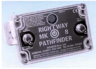
The Portable Rightway Pathfinder MK 8 is an instrument for indicating the passage of fault current in overhead 11KV and 33KV power lines. CHANGES AT A **GLANCE** Improved IP rating to IP67 ensures weatherproofing during prolonged use. Sealed switches (without rubber over-boots) gives this improved IP rating. Modern PIC selection allows zero standing current when alarmed
